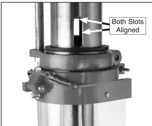
Figure 32. Both drift key slots aligned.
